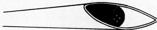
Fig. 2. Tip of the needle electrode showing the plane of the exposed electrode wires.
